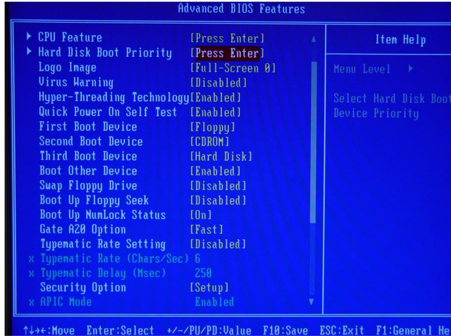
9. Confirm that the USB flash device is the first device the DVN uses to boot, and press **<F10>**.
